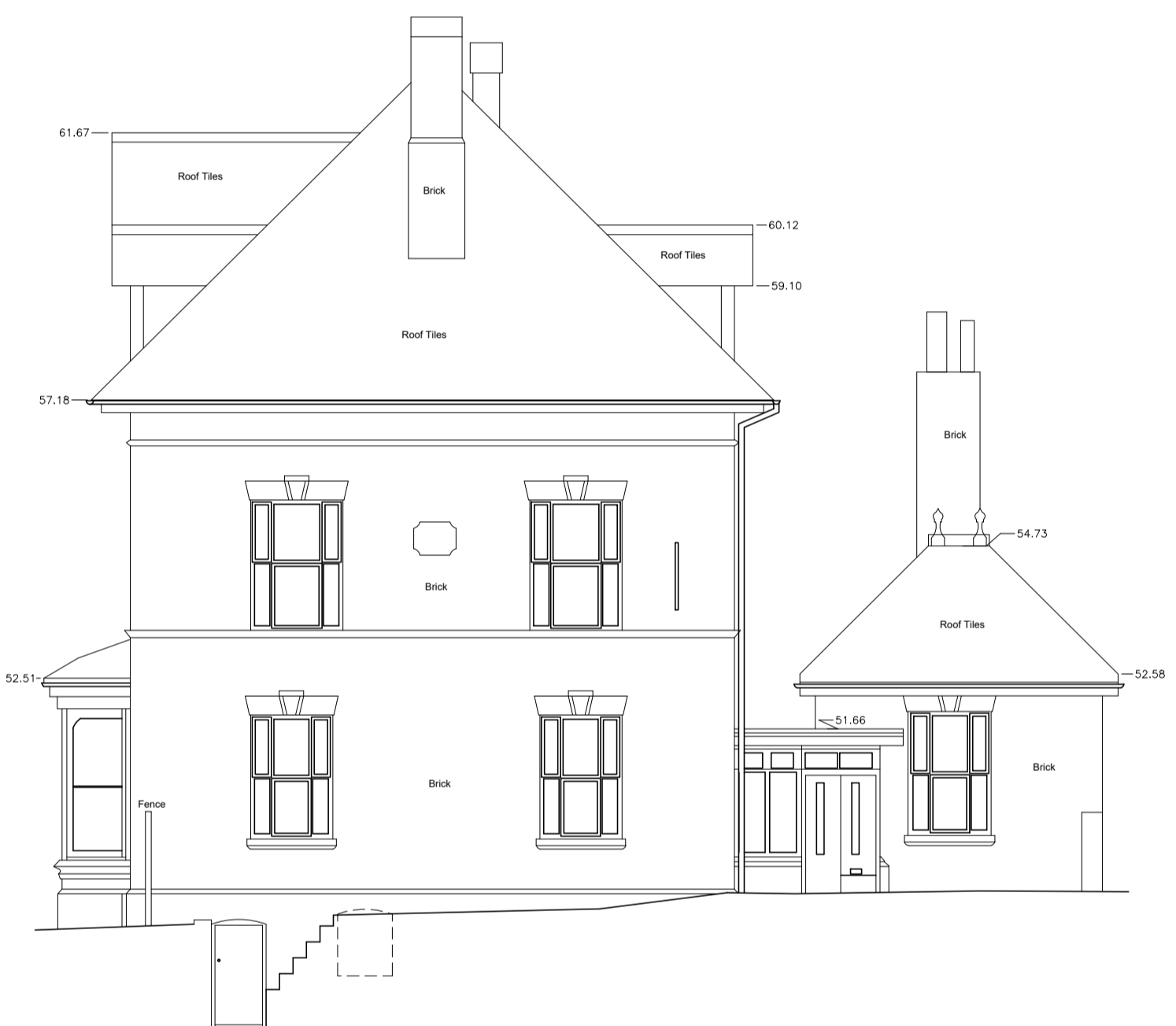
EXISTING FRONT ELEVATION (HIGHWAY FACING) SCALE 1/100
